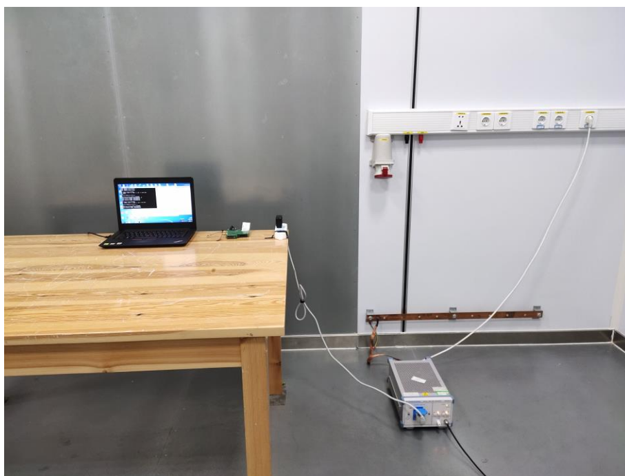
Fig. 4 Power line conducted emission setup photo
