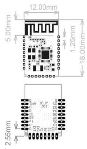
**Note**: The default outline dimension tolerance is  $\pm 0.35$  mm, and the critical dimension tolerance is  $\pm 0.1$  mm.
