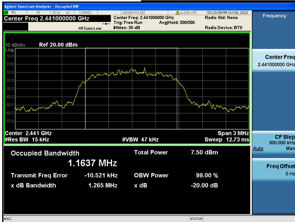
**20 dB BW****Highest Channel & Modulation : 8DPSK**
