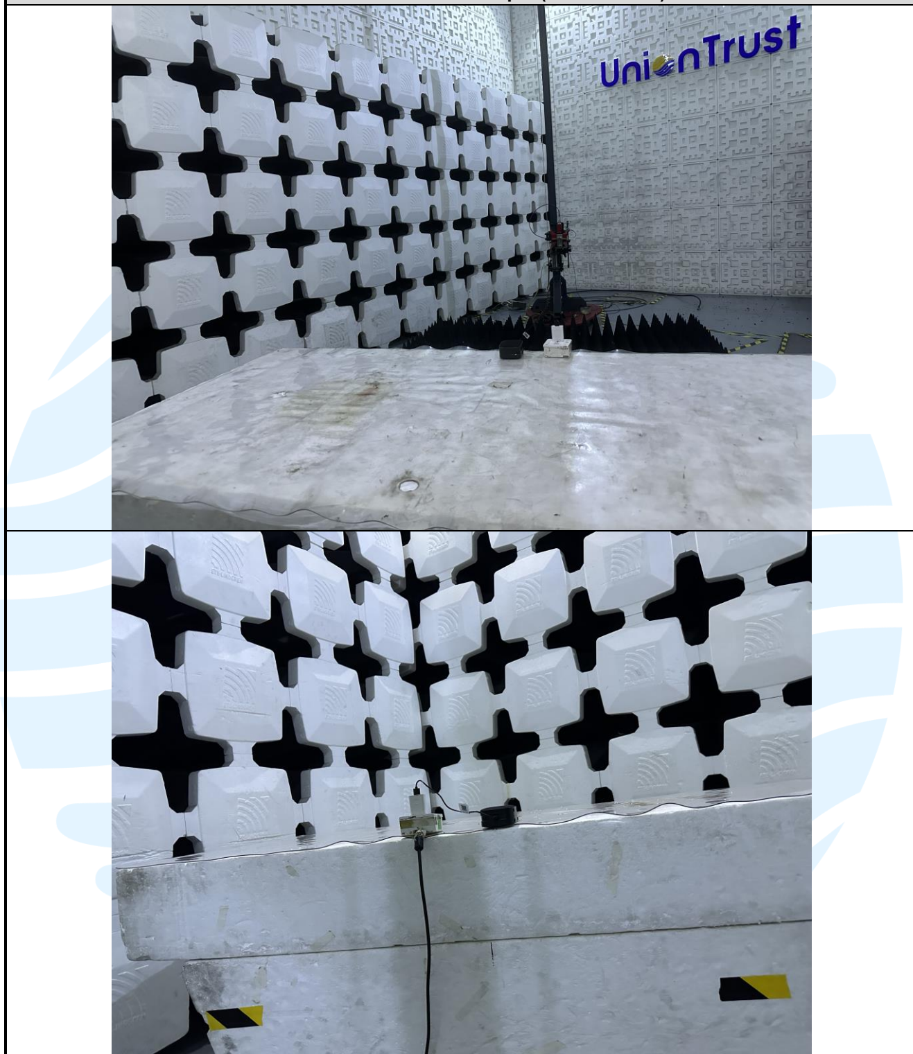
Radiated emission Test Setup-2 (Above 1 GHz)
