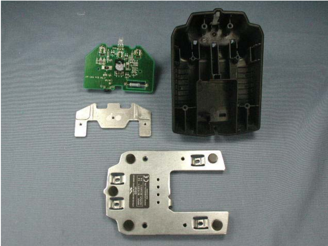
Inside of Battery charger
