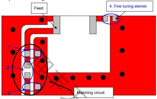
b. Matching circuit: (Center frequency is about 2442 MHz @ 80 x 40 mm² ground plane)
