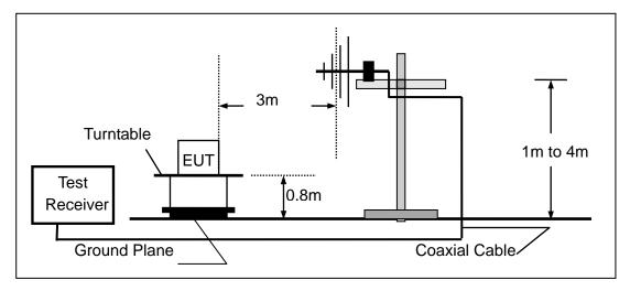
(c) For radiated emissions above 1000MHz
