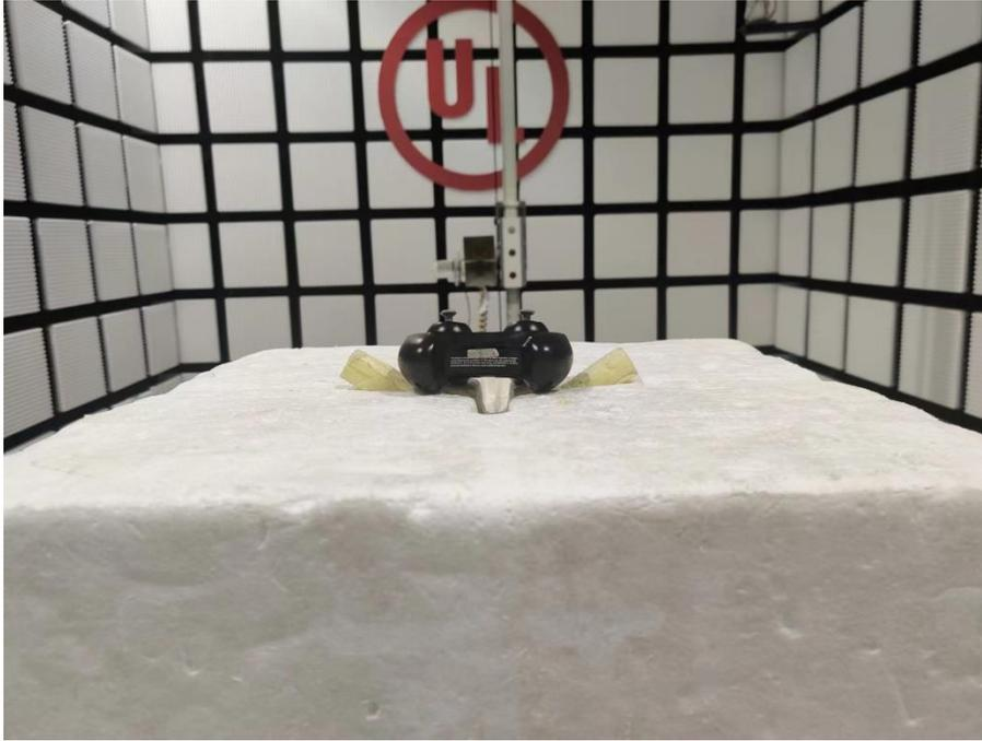
Radiated Disturbance Setup (Above 1 GHz – Y axis)
