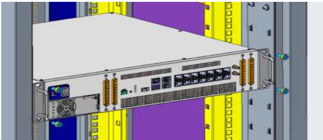
Figure 33. Installation Diagram of DCU in the Rack
