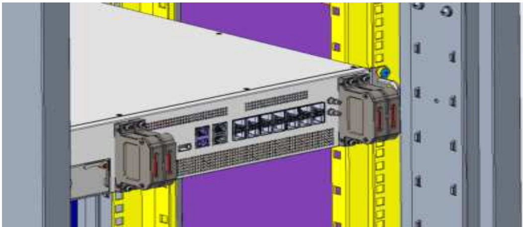
Figure 34. DCU RF Cable Plug Installation
