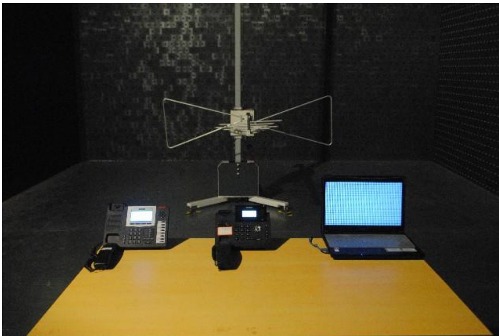
Radiated emission test view (30MHz~1GHz)
