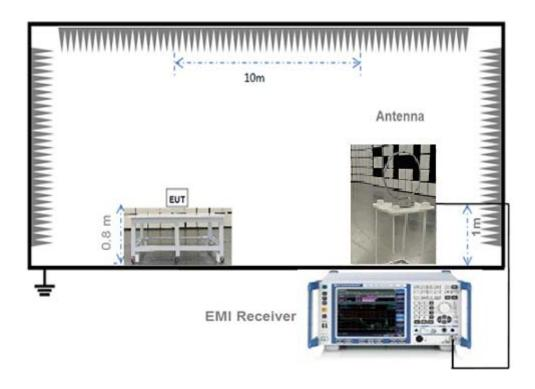
For Radiated Emission Test (Below 30 MHz))
