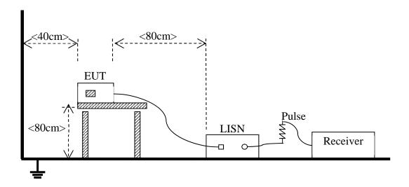
(For Conducted Emission, AC Ports Test)
