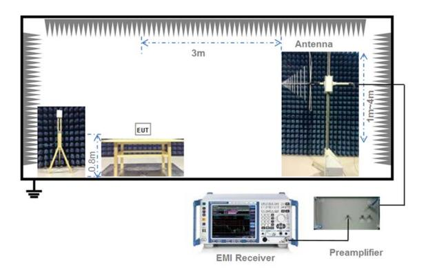
(For Radiated Emission Test (30 MHz-1 GHz))
