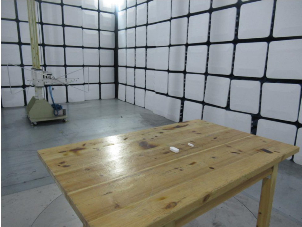
Photo of Radiated Emission Measurement
