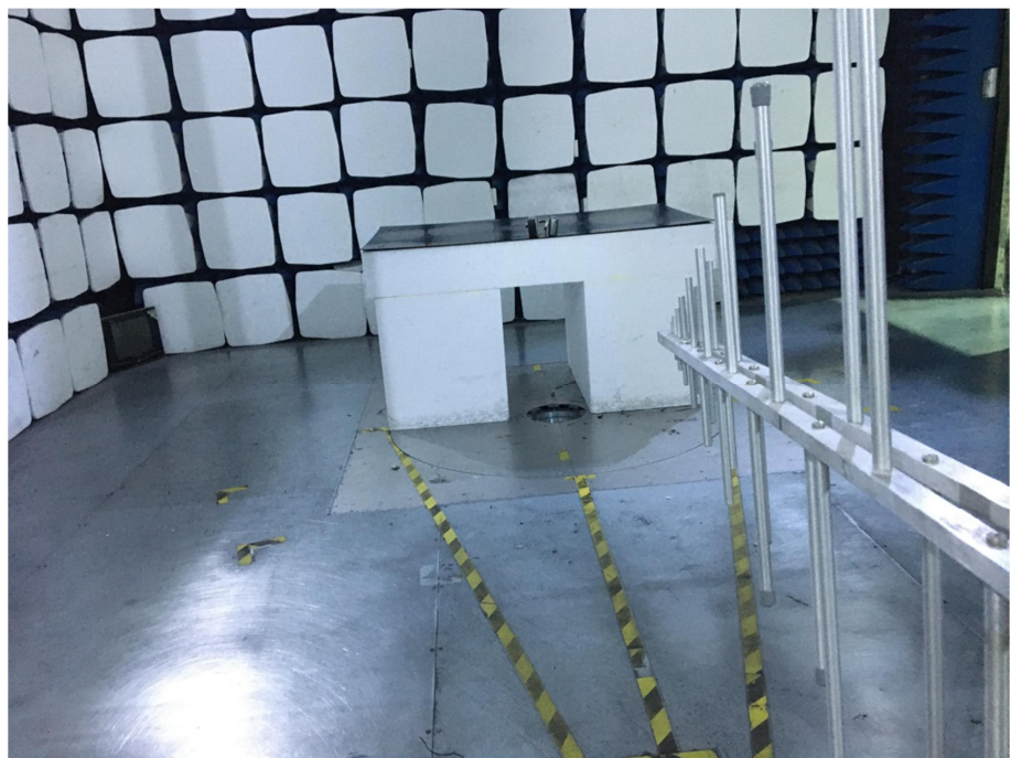
Radiation Emission Test Setup (30MHz to 1GHz)
