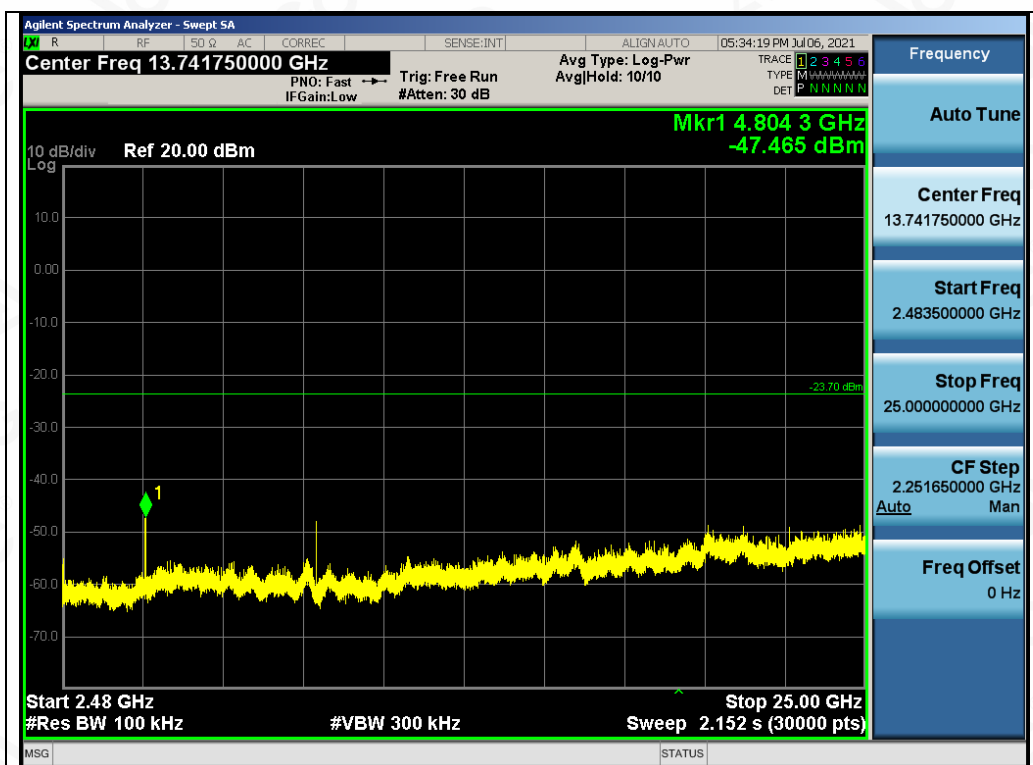
Test_Graph_BR_ANT1_2402_1Mbps_Higher Band Emissions
