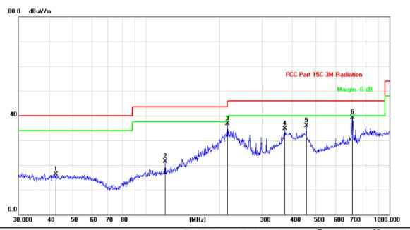
Site Polarization: Horizontal Temperature: 25
