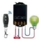
3. Technicalindicators Input voltage: 90V-264V OUtput current: 30A RF Working frequency, 433MHz Range: up to 100 rn in open field Receiver Sensitivity: -95dbm Max number or controllers: 16
