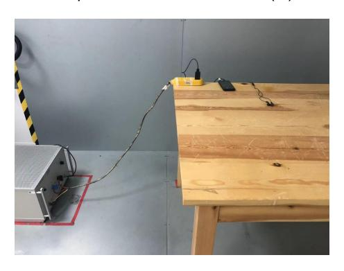
Set-up for Radiated Emission (RE), Below 1GHz
