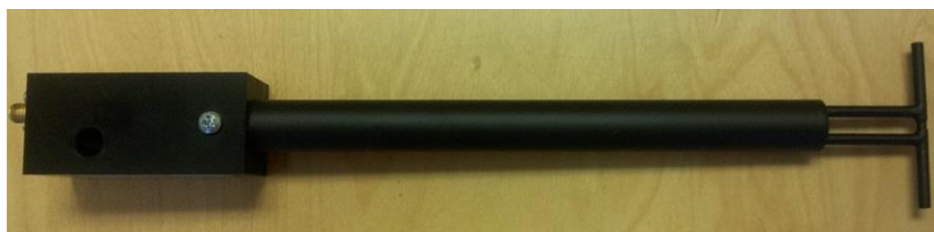
Figure 1 – MVG COMOSAR Validation Dipole
