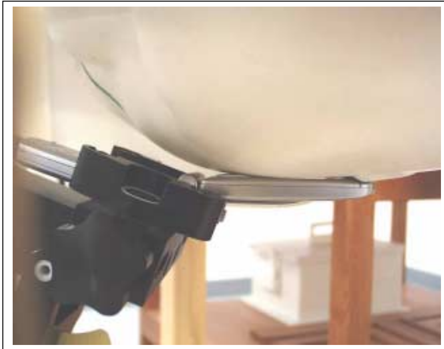
EUT Setup Configuration 1 (Left Head - Tilted position)
