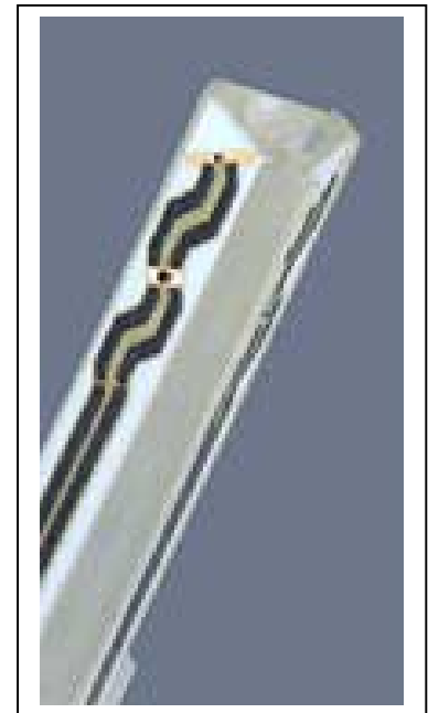
Inside view of ET3DV6 E-field Probe
