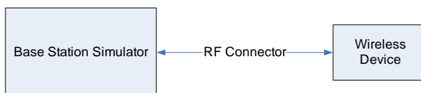
Figure 9-1 Power Measurement Setup
