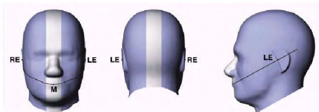
Figure 5-2 Front, back and side view of SAM Twin Phantom
