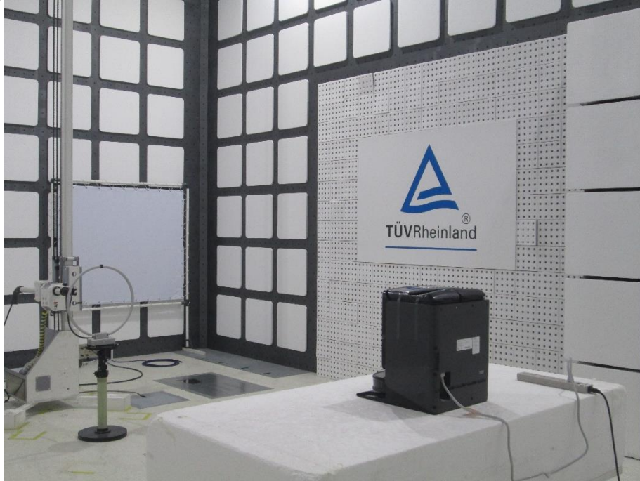
Photograph 4: Test Setup for Spurious Emissions (Back View 2)
