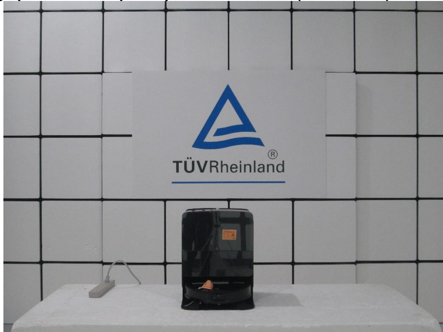
Photograph 2: Test Setup for Spurious Emissions (Front View 2)
