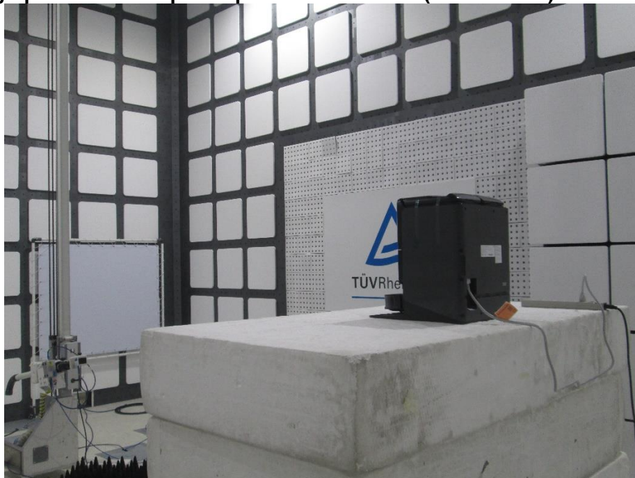
Photograph 6: Test Setup for Spurious Emissions (Back View 4)
