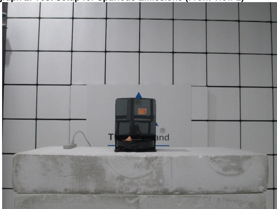
Photograph 2: Test Setup for Spurious Emissions (Front View 2)
