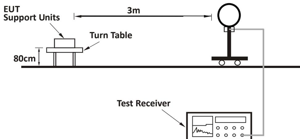
**For Radiated emission 30MHz to 1GHz:**
