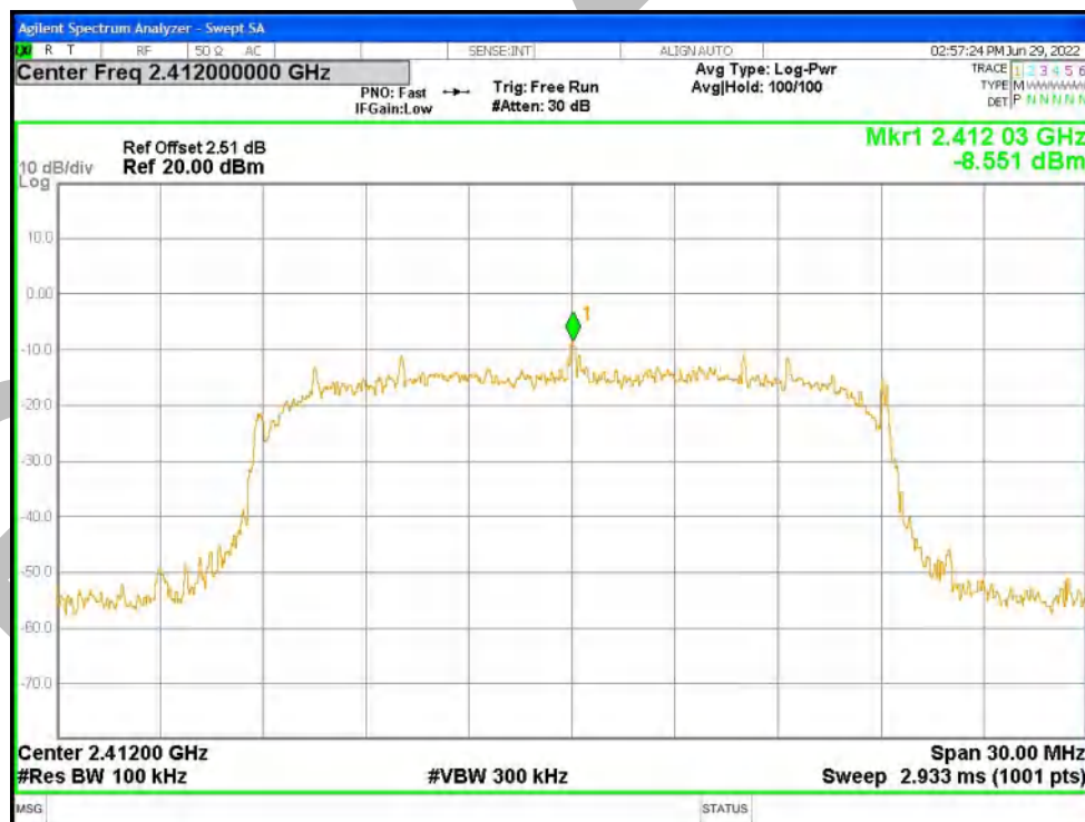
Tx. Spurious NVNT n20 2412MHz Ant1 Emission
