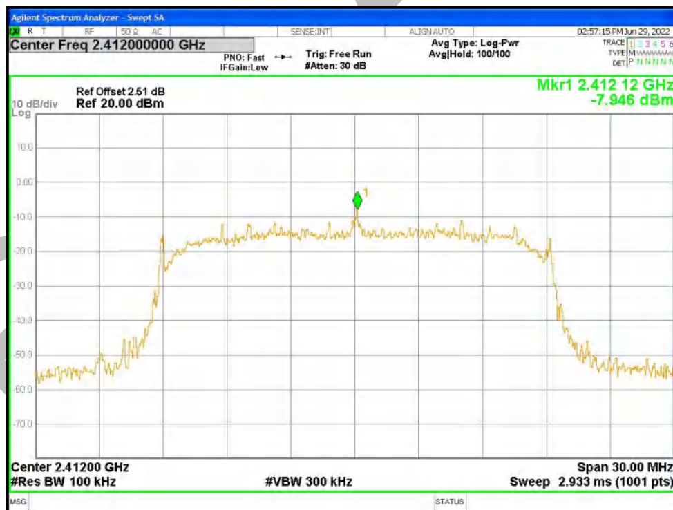
Band Edge NVNT n20 2412MHz Ant1 Emission
