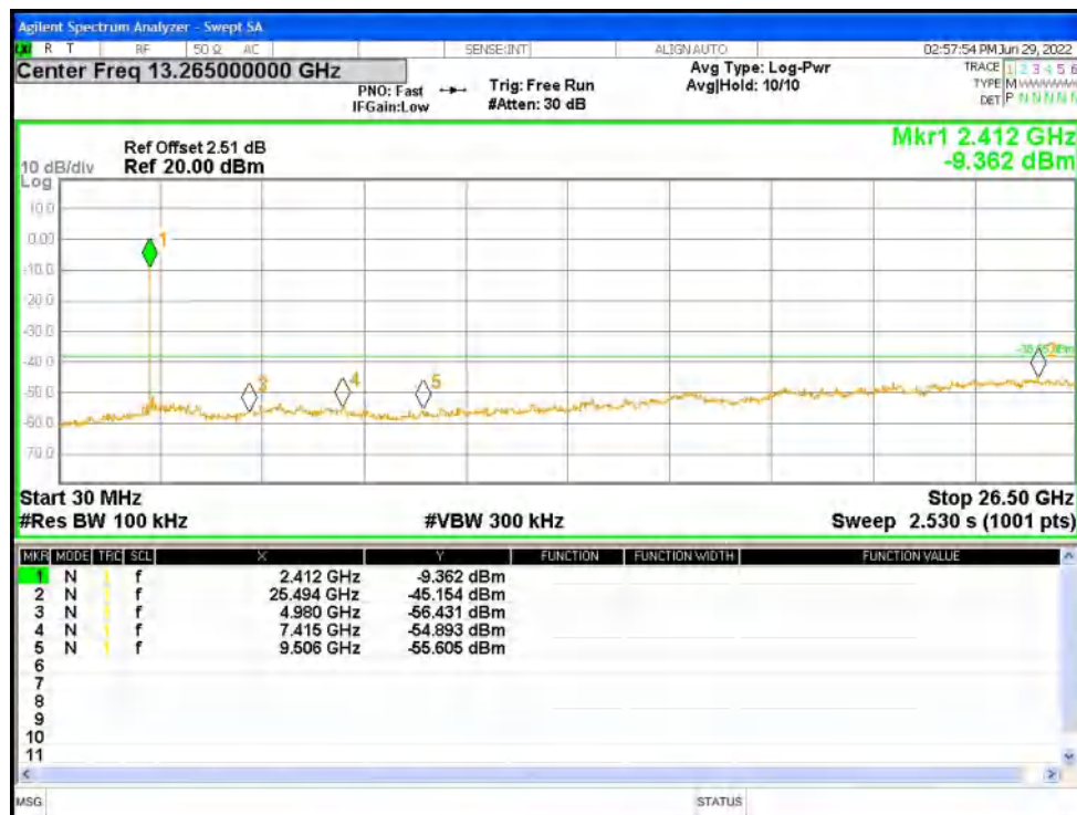
Tx. Spurious NVNT n20 2437MHz Ant1 Ref
