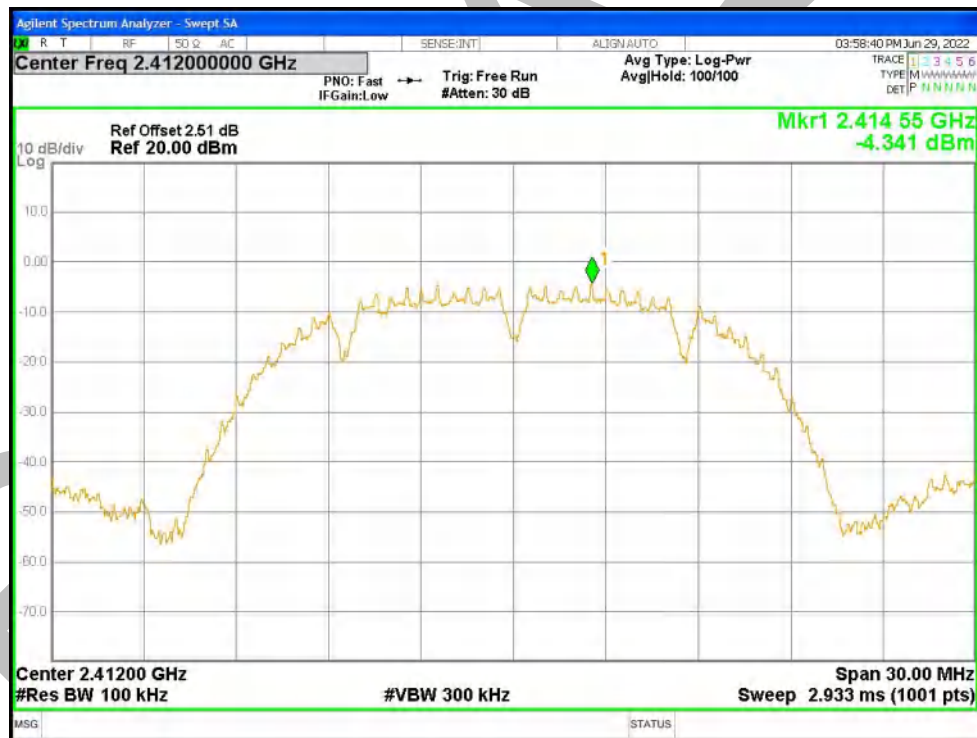
Tx. Spurious NVNT b 2412MHz Ant1 Emission
