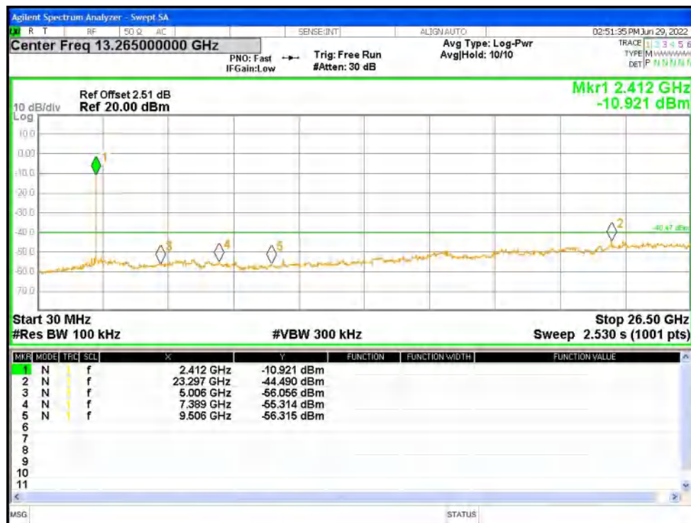
Tx. Spurious NVNT g 2437MHz Ant1 Ref
