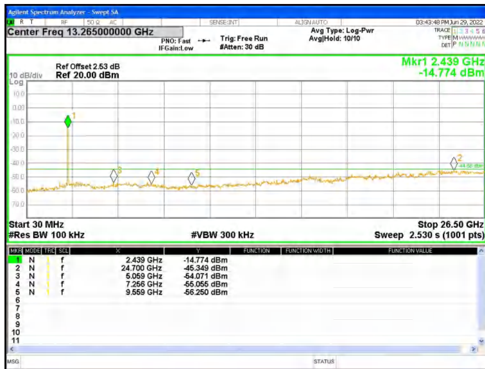
Tx. Spurious NVNT n40 2452MHz Ant1 Ref
