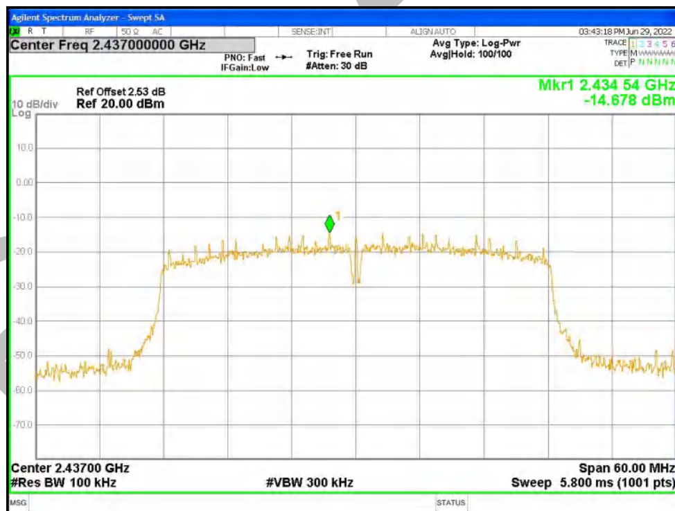
Tx. Spurious NVNT n40 2437MHz Ant1 Emission
