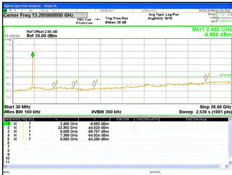
Tx. Spurious NVNT n20 2412MHz Ant1 Ref
