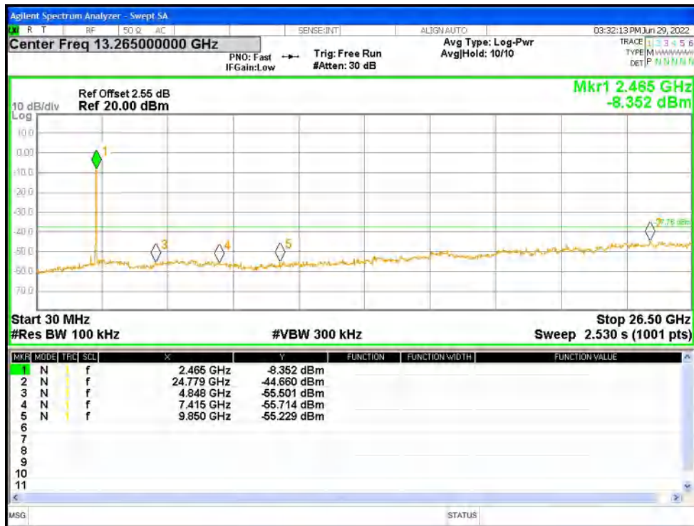
Tx. Spurious NVNT n40 2422MHz Ant1 Ref
