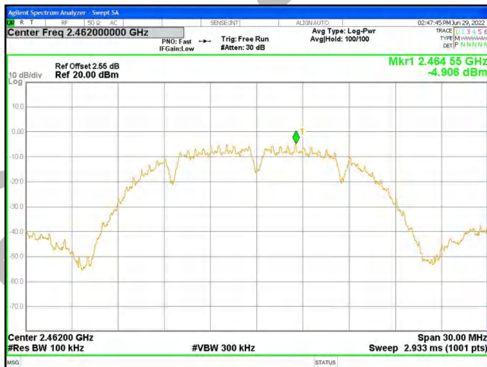
Band Edge NVNT b 2462MHz Ant1 Emission
