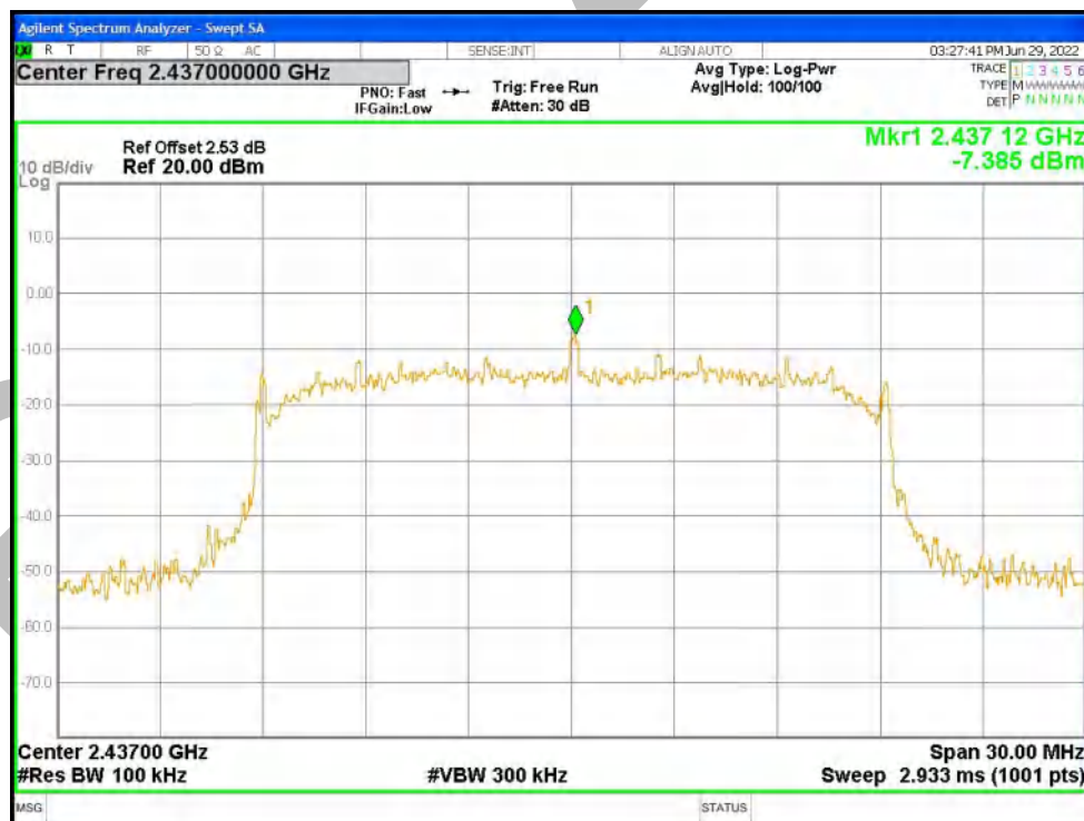
Tx. Spurious NVNT n20 2437MHz Ant1 Emission
