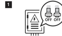
ENSURE THAT YOU HAVE TURNED OFF ALL POWER TO DOORBELL WIRING AT YOUR BREAKER BOX. If using power adapter, ensure that the adapter is UNPLUGGED.
