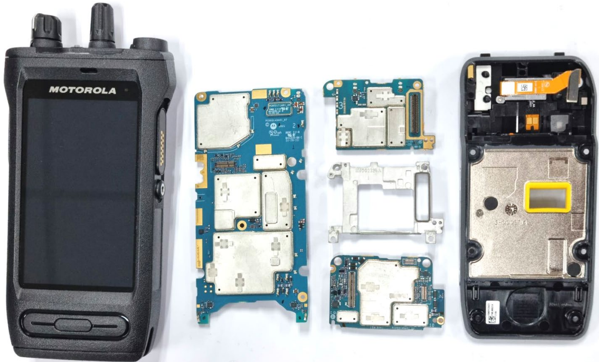
Exhibit 9M: RF boards with chassis and housing for (Front Side)
