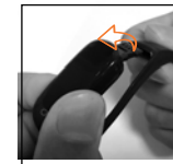
3. Pull out the USB charging interface.
