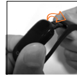
5. Insert the USB charging interface.
