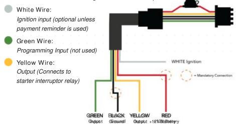
Once the wires are attached and Evo is mounted, plug the harness into it and power up.
