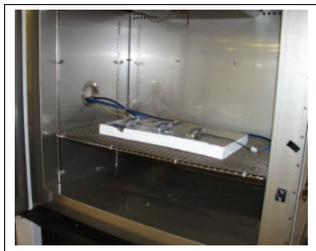
Fig. 3: Frequency Stability Setup
