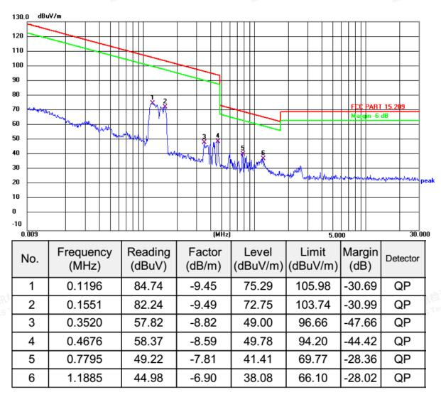
Remark: 1). Measured at antenna position 0 degree and 90 degree, recorded worst case at 0 degree. 2). Margin=Reading level + Factor- Limit.
