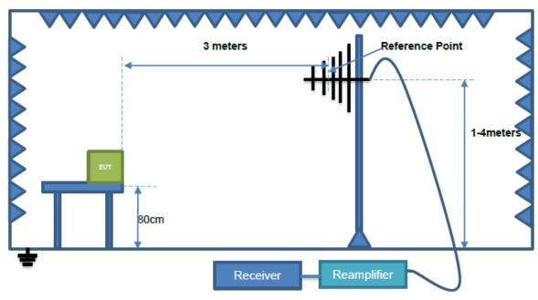
Radiation Test (30MHz - 1GHz)
