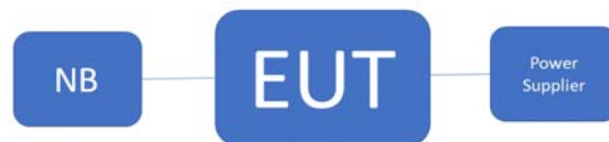
Fig. 2-2 Conducted (Antenna Port) Configuration
