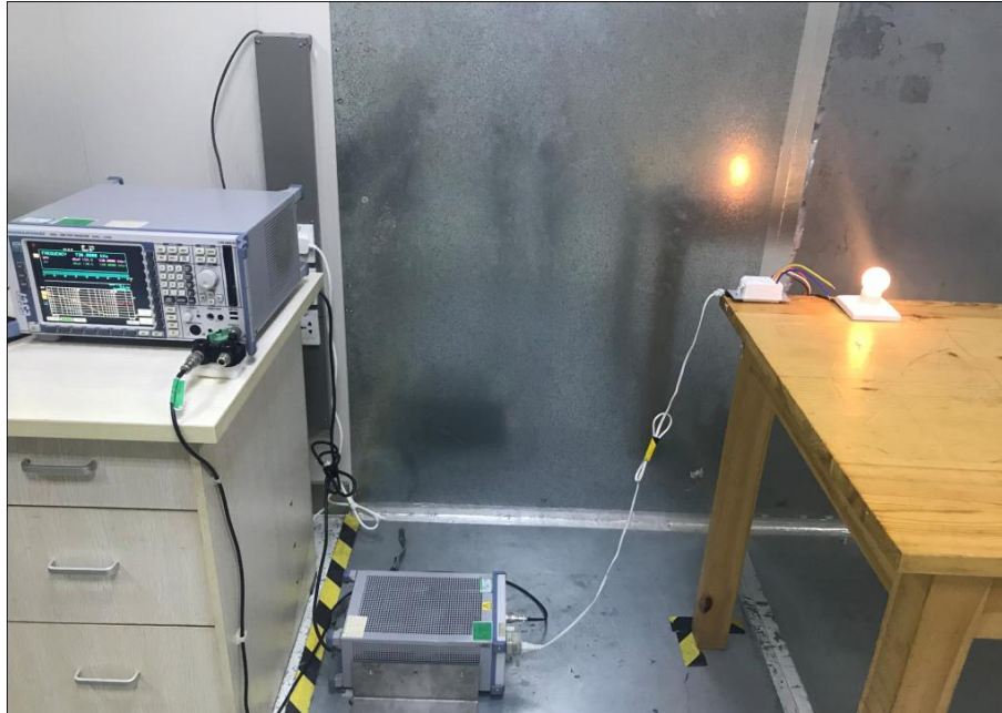
Radiated Spurious Emissions Test Frequency From 30MHz-1000MHz
