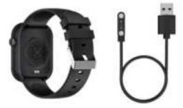
Align the charging head and fit the magnetic charging port until the charging icon appears on the watch screen (continuous charging with a 5V charging head for 2-3 hours).
