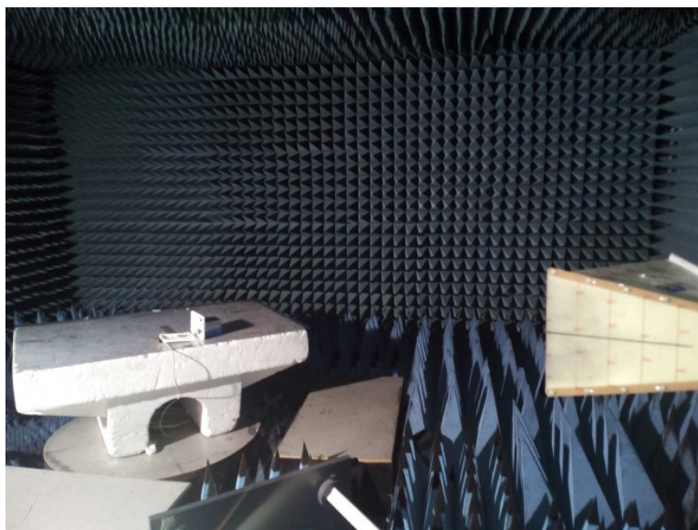
Photograph 8.1.3 Setup for radiated emission measurements, EUT cabling
