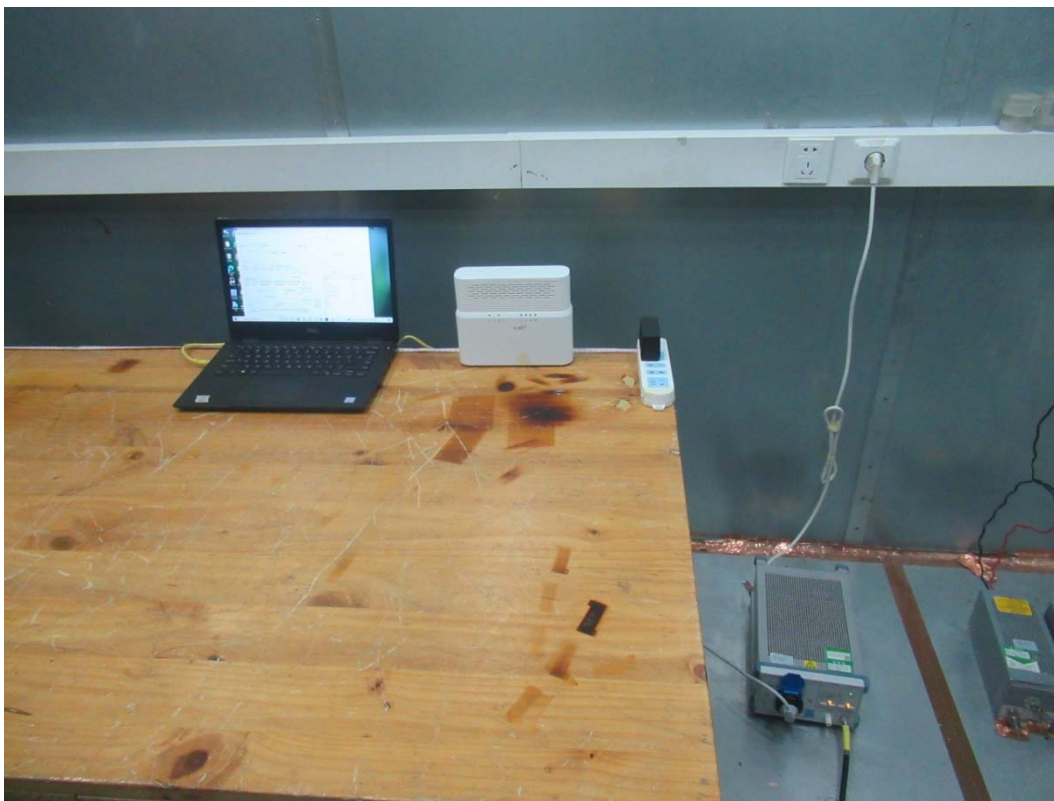
Picture 2 Conducted Emission Test Setup
