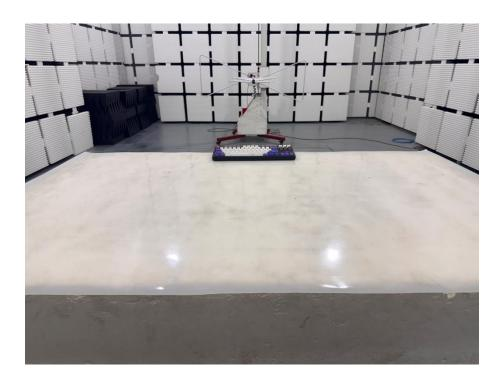
Set-up for Radiated Spurious Emission, Above 1GHz
