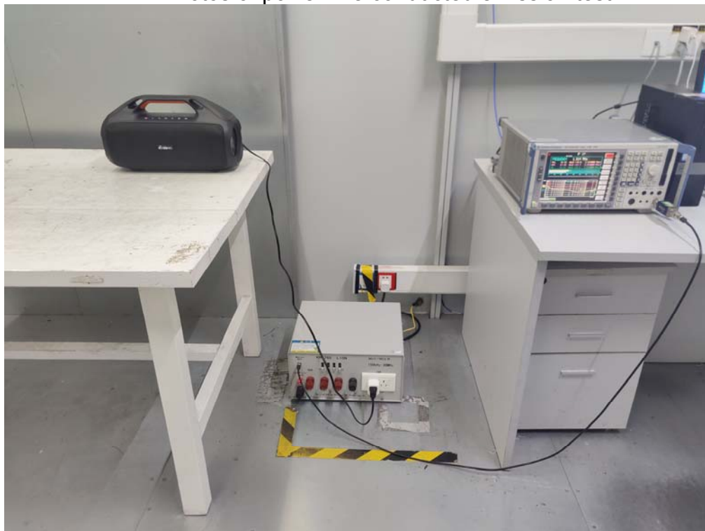
Photos of power line conducted emission test
