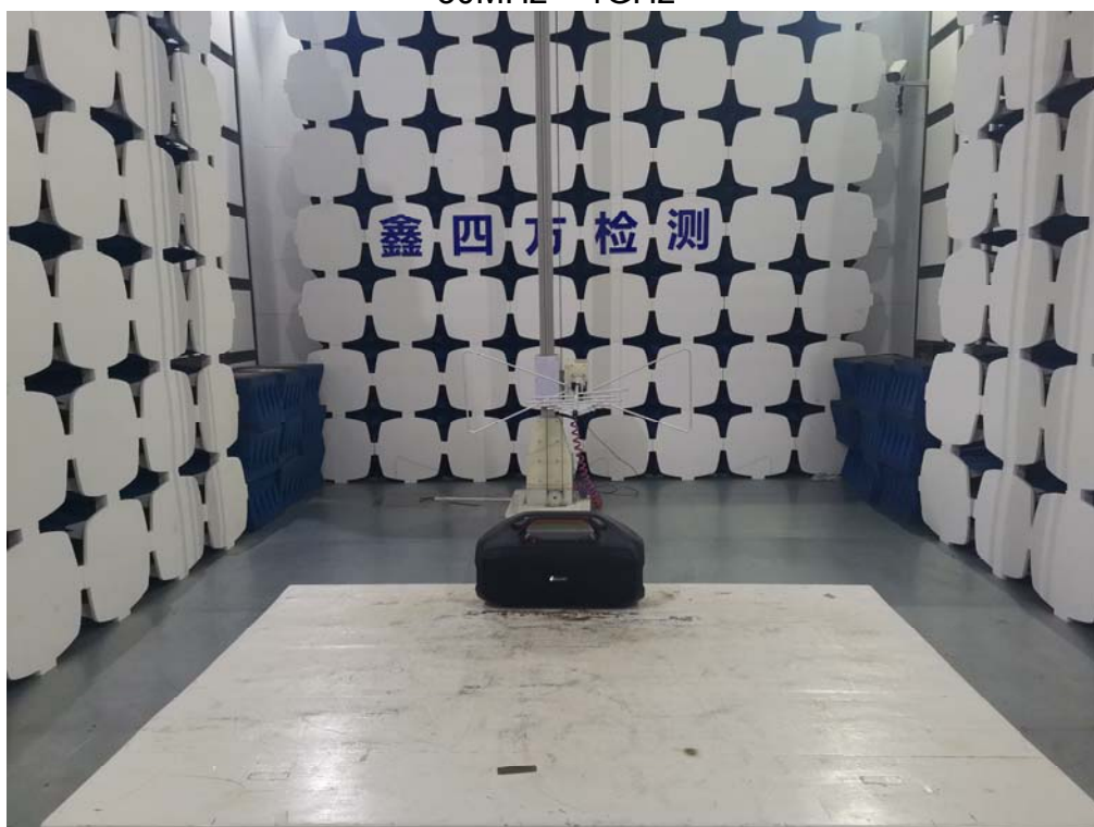
Photos of radiated emission test 30MHz – 1GHz
