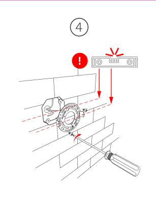
Secure the bracket to the outlet box with the screws.
