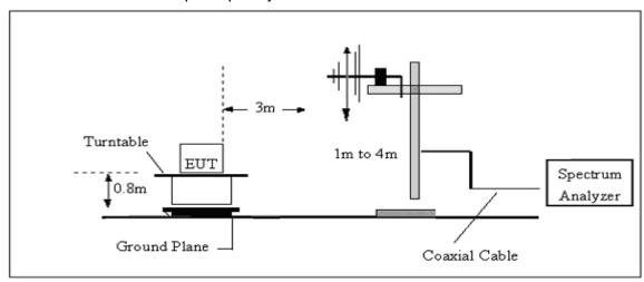
3. Radiated Emission Test-Up Frequency Above 1GHz
