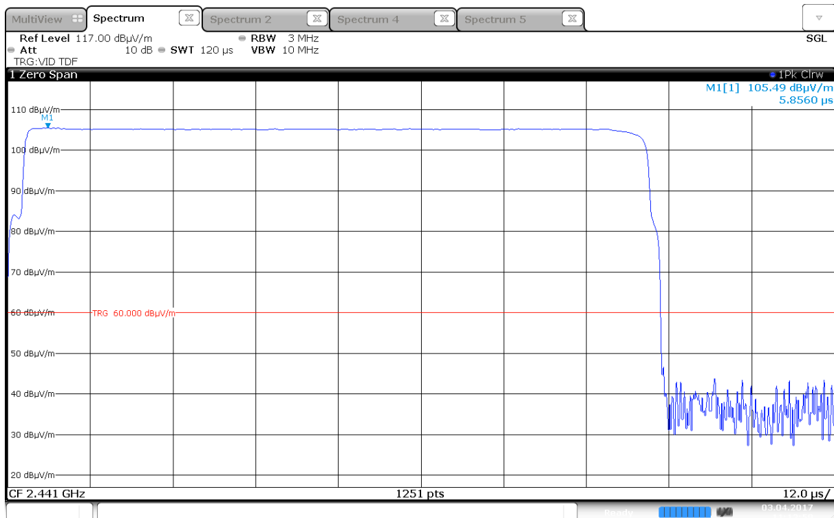
Radiated Power, 2441 MHz (Max: Ant2, VP)
