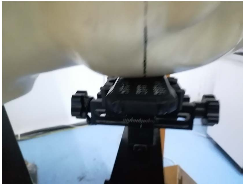
Head Left Cheek Setup Photo (0mm)
