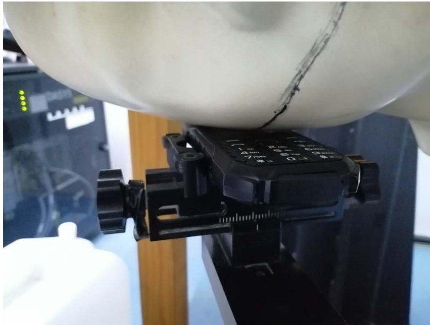
Head Right Tilt Setup Photo (0mm)
