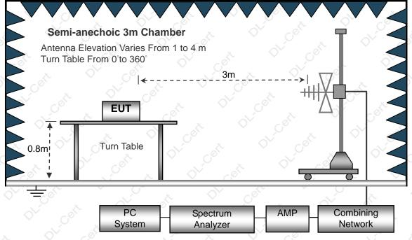
(C) Radiated Emission Test-Up Frequency Above 1GHz
