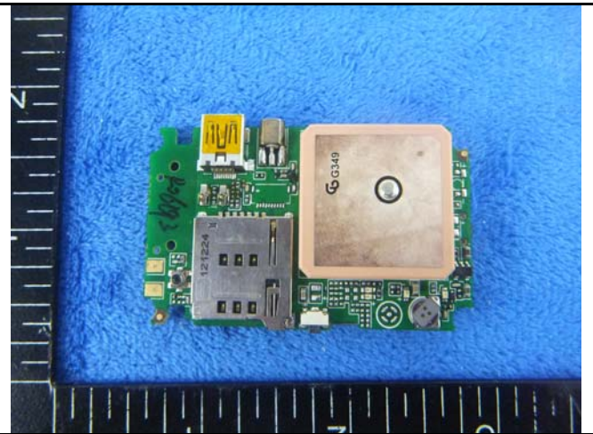
Mainboard Without Shielding - Front View
