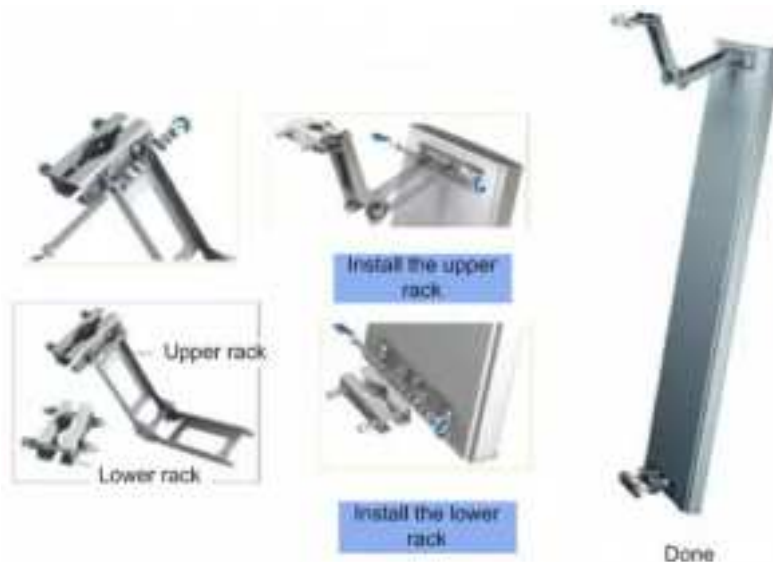
Figure 3-6 Assembling Procedure of Directional Antennas
