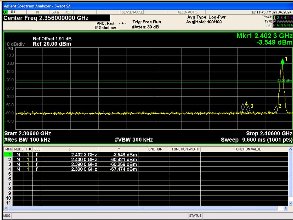
Test Model PSD(Power Spectral Density ) RBW=100kHz
