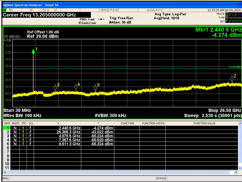
**PSD(Power Spectral Density ) RBW=100kHz**
