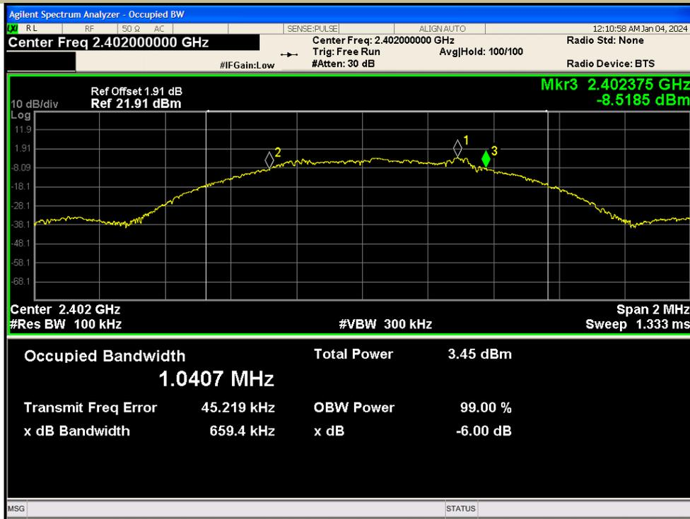
Test Model DTS (6dB) Bandwidth
