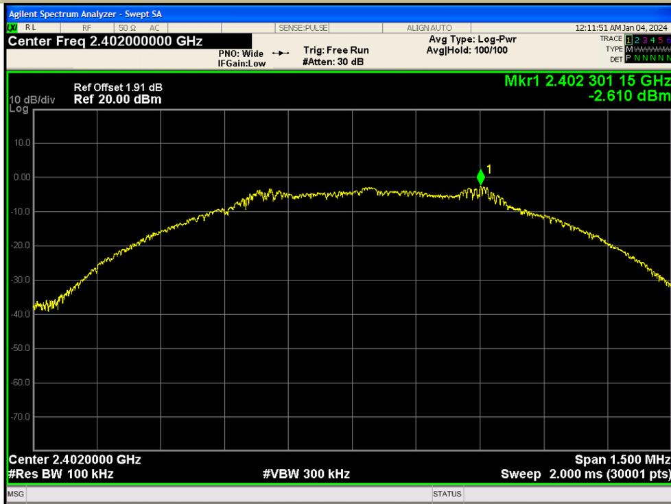
Test Model Unwanted Emissions in non-restricted frequency bands
