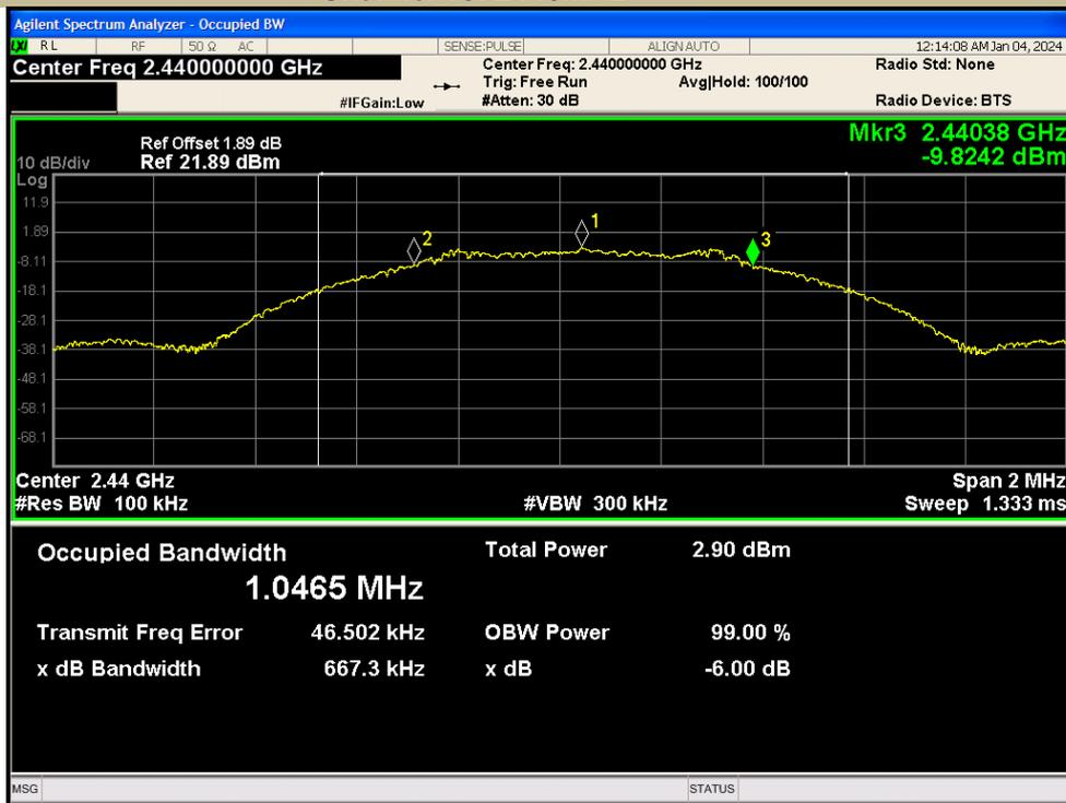
Test Model DTS (6dB) Bandwidth
