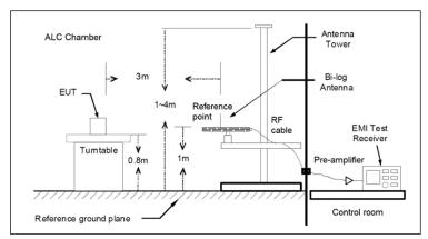
Radiated measurements setup f > 1-18 GHz
