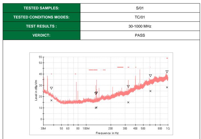
PK+\_MAXH TX limits to Spurious Emission FOC15.247 (30MHz to 1 GHz) Restricted Bands QPK Limit MaxPeak-PK+ (Single) QuasiPeak-QPK (Single)
