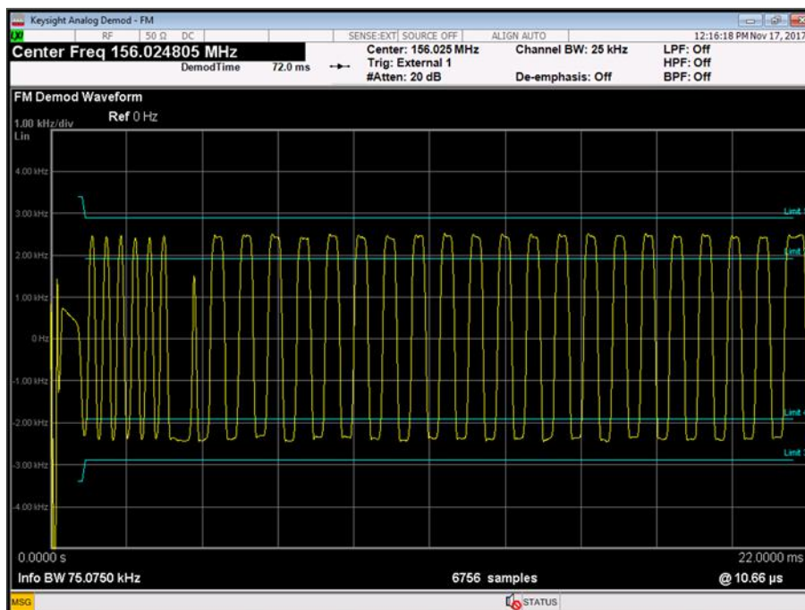
Figure 17 - 156.025 MHz, Test Signal #2, Tx2, -15.0 °C, 9.6 V DC
