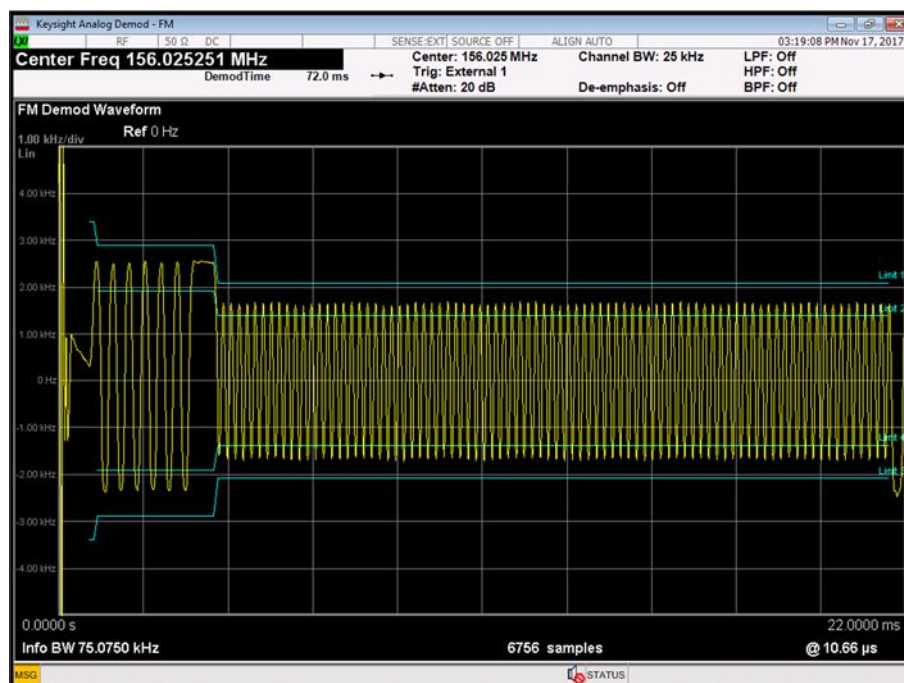
Figure 22 - 156.025 MHz, Test Signal #1, Tx1, +55.0 °C, 31.2 V DC
