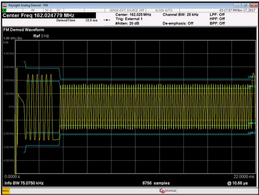
Figure 27 - 162.025 MHz, Test Signal #1, Tx2, +55.0 °C, 31.2 V DC
