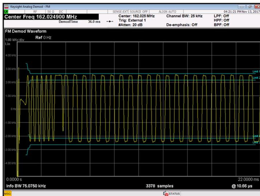
Figure 12 - 162.025 MHz, Test Signal #2, Tx1, +21.9 °C, 12.0 V DC
