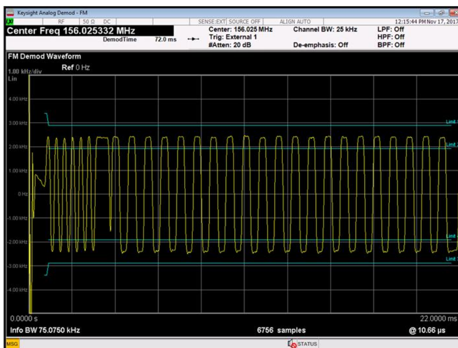
Figure 16 - 156.025 MHz, Test Signal #2, Tx1, -15.0 °C, 9.6 V DC
