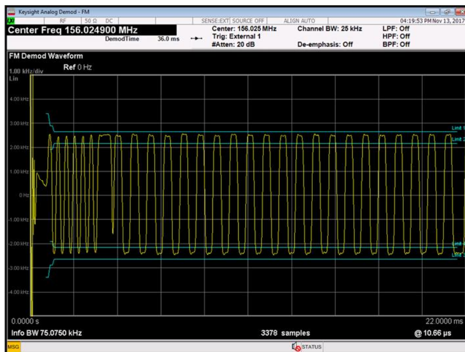
Figure 8 - 156.025 MHz, Test Signal #2, Tx1, +21.9 °C, 12.0 V DC
