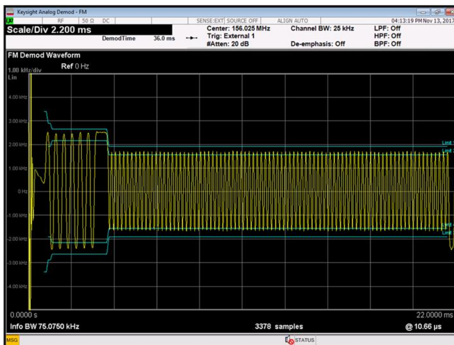
Figure 6 - 156.025 MHz, Test Signal #1, Tx1, +21.9 °C, 12.0 V DC
