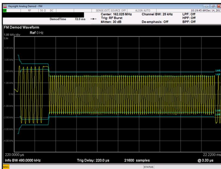
Figure 10 - 162.025 MHz, Test Signal #1, Tx1, +21.9 °C, 12.0 V DC
