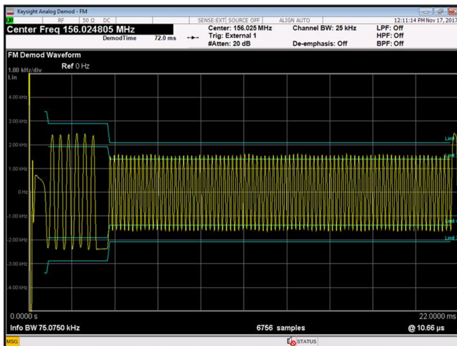
Figure 15 - 156.025 MHz, Test Signal #1, Tx2, -15.0 °C, 9.6 V DC
