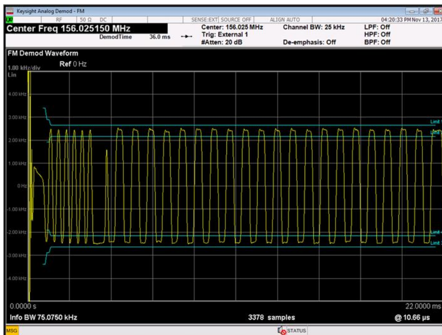
Figure 9 - 156.025 MHz, Test Signal #2, Tx2, +21.9 °C, 12.0 V DC
