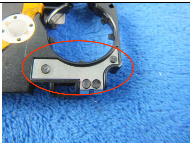
WIFI - Antenna View
