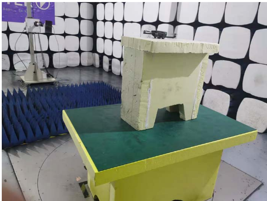
Spurious Emission Test Setup (Above 1GHz)
