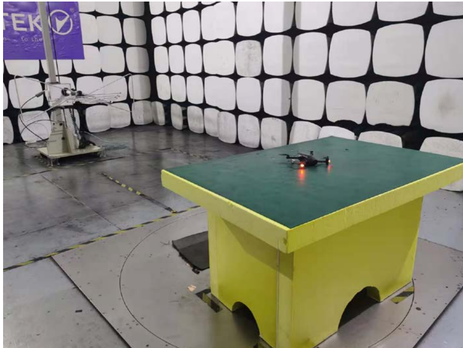
Spurious Emission Test Setup (Below 1GHz)
