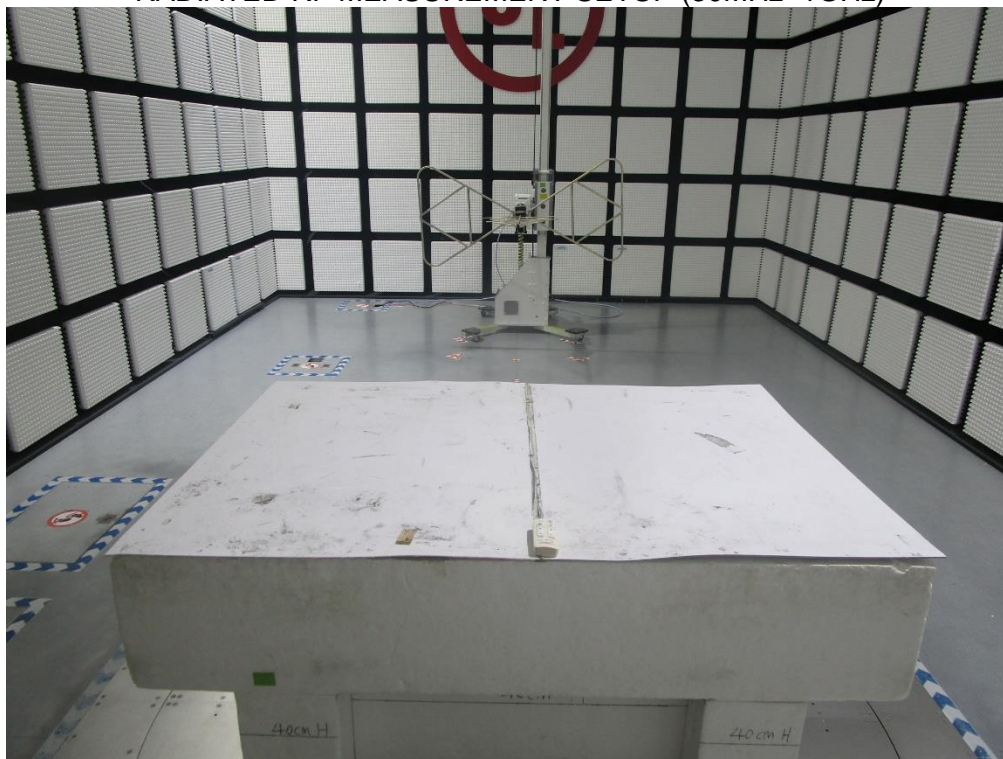
RADIATED RF MEASUREMENT SETUP (Below 30MHz)
