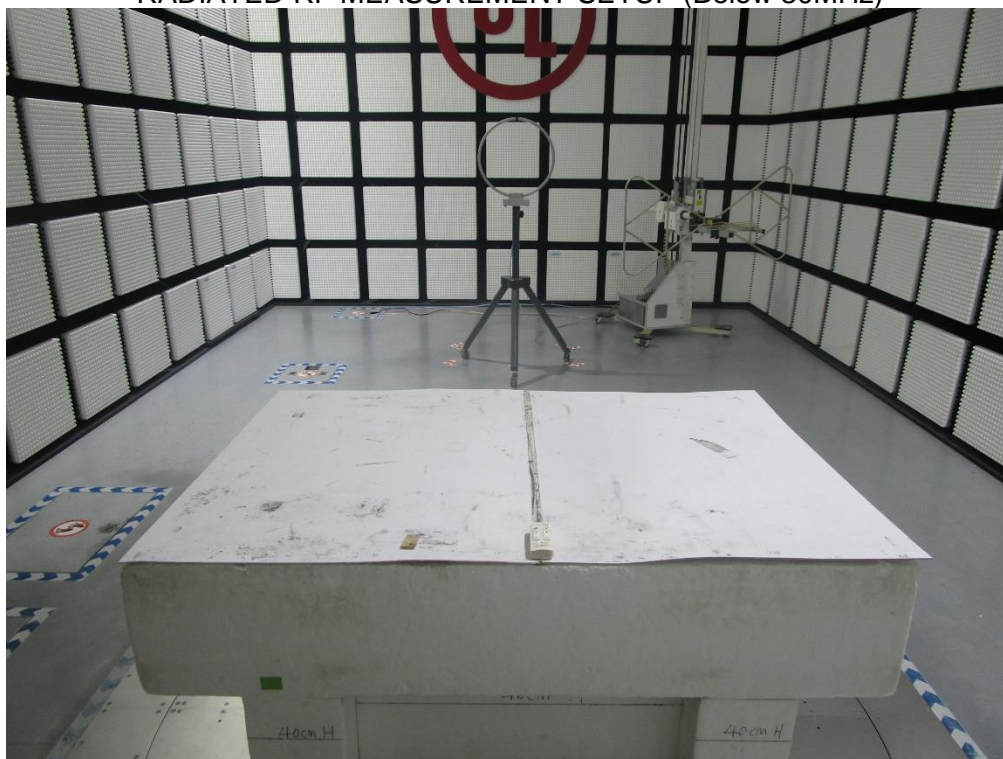
RADIATED RF MEASUREMENT SETUP (Below 30MHz)
